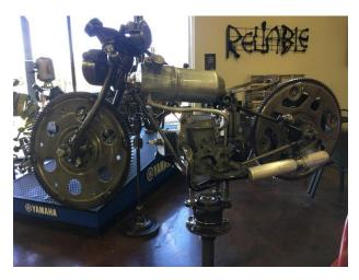
Pedestal – rear brake drum, axle, rear differential ring gear, bearing race, hub assembly
